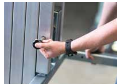
Assembly and fixing of the Load fork using ball lock pins
