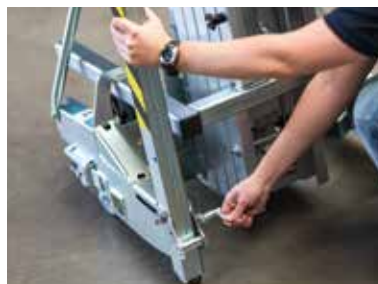
Opening and fixing of front sections by means of spring locking bar
